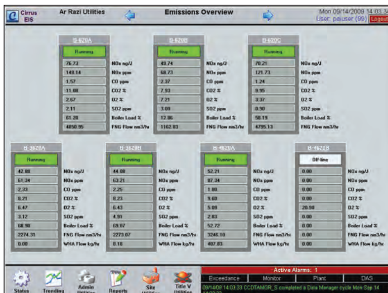
FIGURE 6. The summary status of all crucial boiler parameters can be displayed on one page
