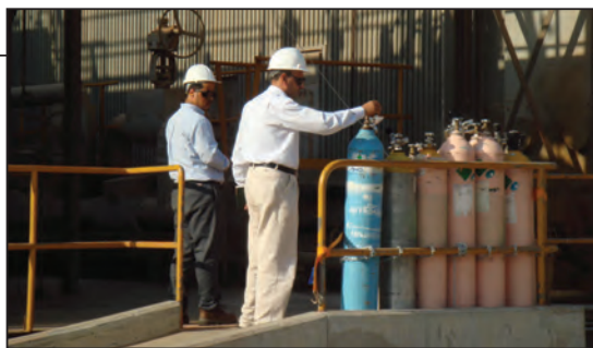
FIGURE 4. An onsite PEMS inspection and relative accuracy test audit (RATA) were conducted by regulatory agencies
